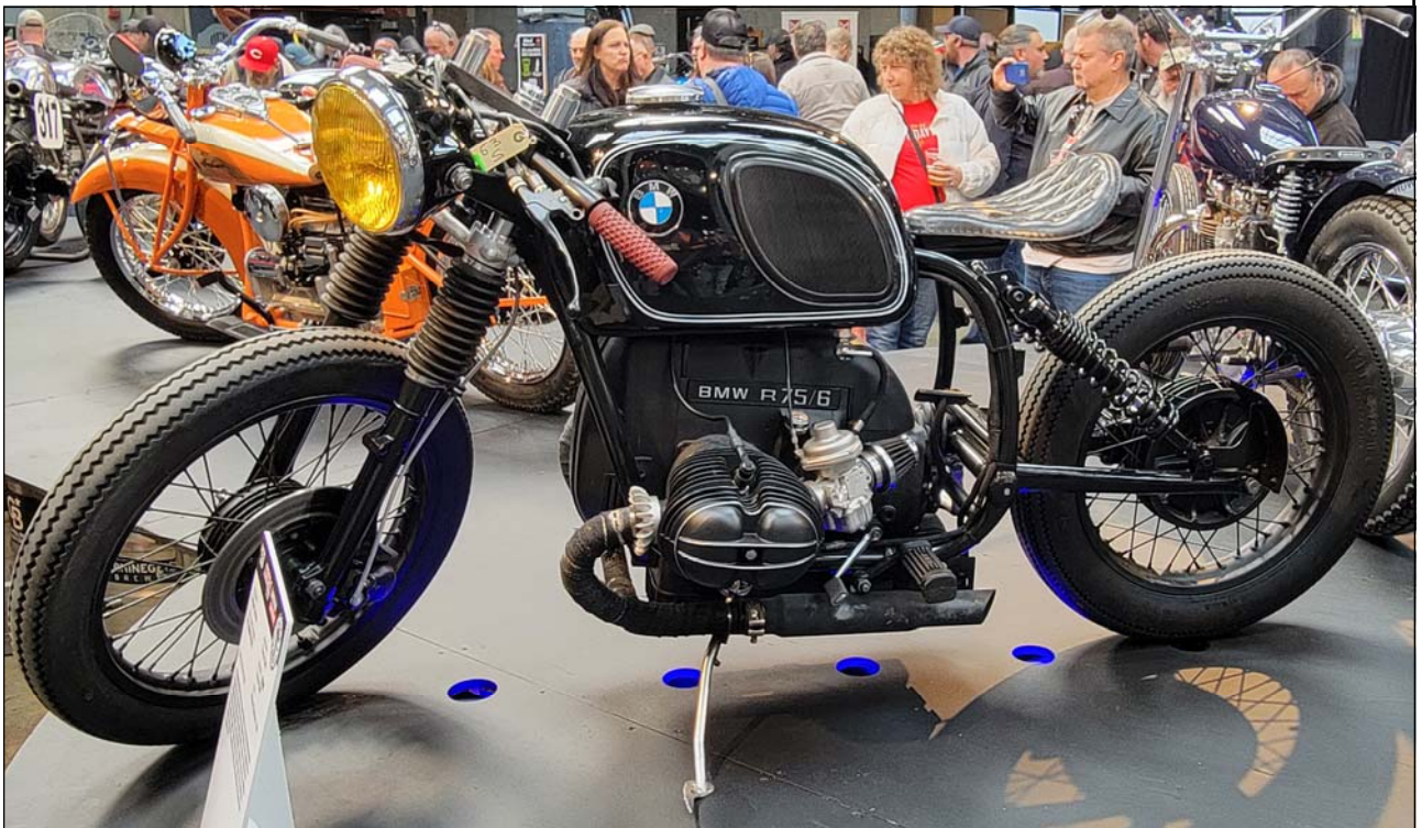
1974 BMW R75/6 Updates include a 1000cc kit, electronic ignition, LED indicator lights built into triple tree, battery relocation, subframe delete and updated front and rear suspension.
