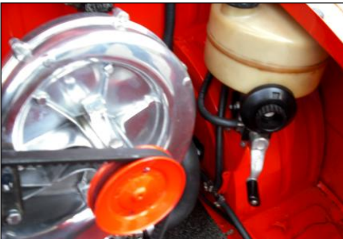
The Vespa 400 employs a twin-cylinder, air-cooled, two-stroke with dual points and a hand pump(right side) to meter an oil mix to the fuel tank (left side of engine compartment).
