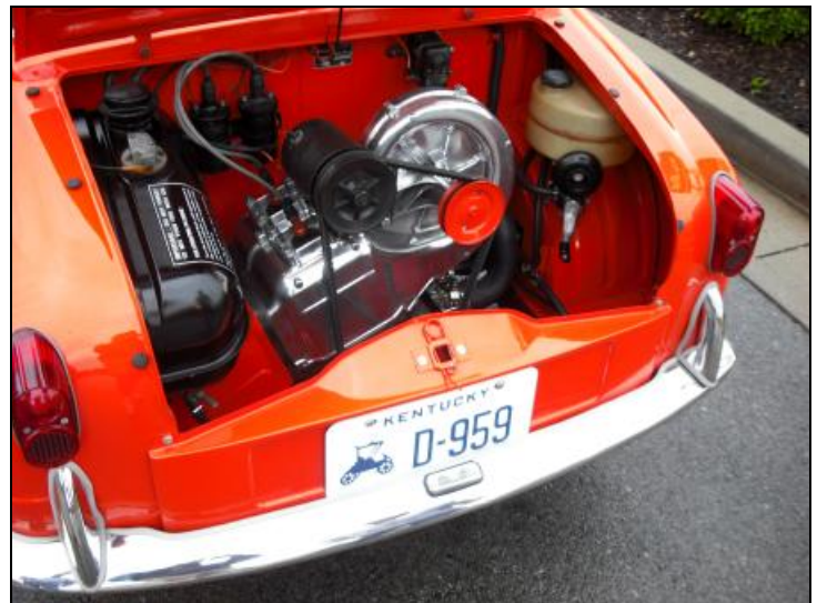
The Vespa 400 employs a twin-cylinder, air-cooled, two-stroke with dual points and a hand pump(right side) to meter an oil mix to the fuel tank (left side of engine compartment).
