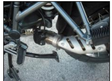
Micatech provides an exhaust pipe adapter that lowers the muffler to enable a full-size bag on the left side of the bike as pictured below.
