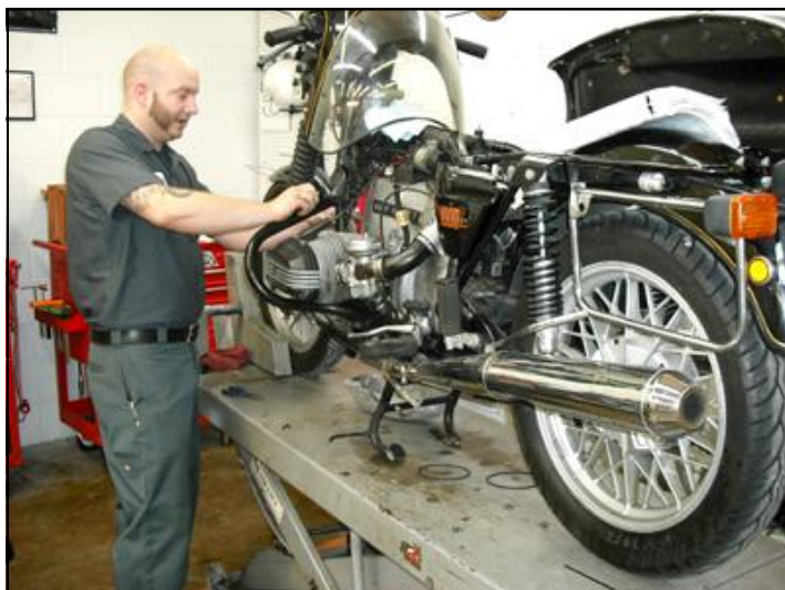
Dean Beatty replaces a diode board on an R100/7.
